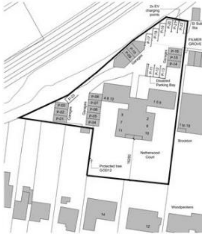
Proposed Block Plan 0 5m 10m 25m 50m scale 1:500
